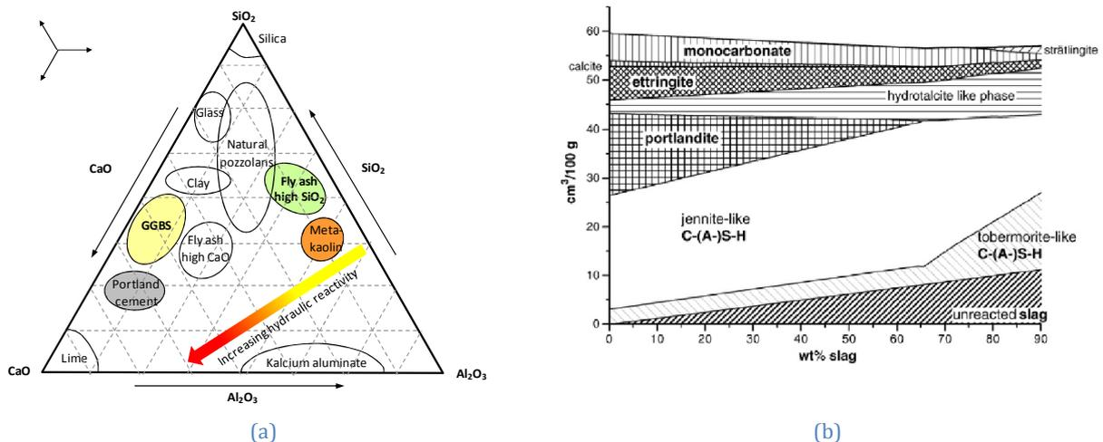
Figure 1. (a) Chemical composition (main components) of cementitious materials. (b) Hydration products with different amounts of GGBS (slag).
